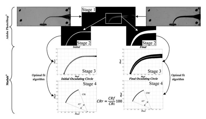
Figure 1. Scheme to determine the CRr parameter.
